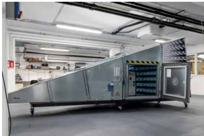
Camera anecoica (EMEA Testing Lab)
